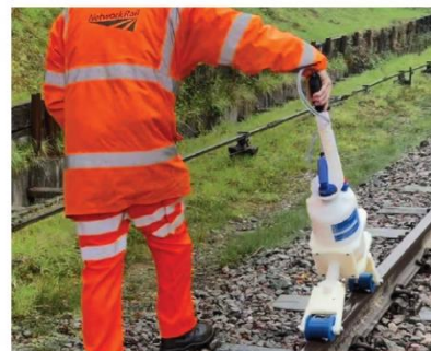
Converted Sand Pram rail head applicator (Blade)
