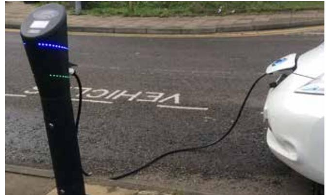
*Electric vehicle plugged into a standalone column charge point. This is on-street, but the principle of a cable to the front of the car is the same for off-street charge points.*
