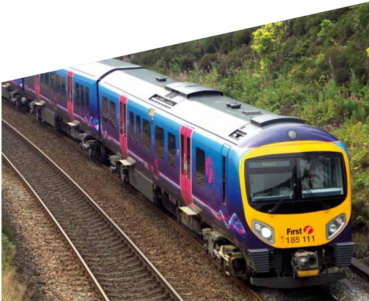
*A Siemens FTPE Type B class 185 'Desiro' DMU of 2005*
