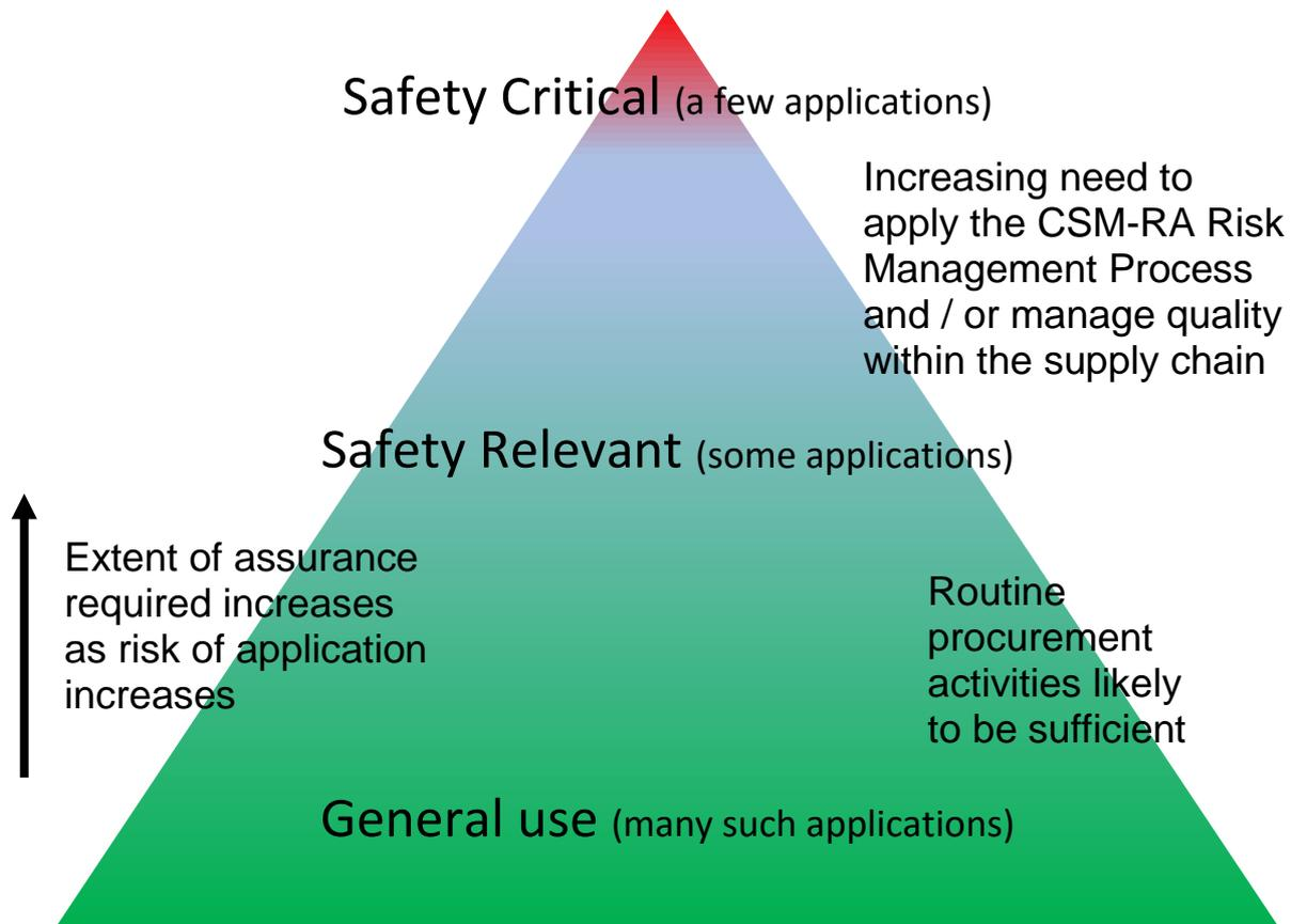
**Figure 1** Diagram illustrating the relative levels of use of fasteners and the extent of risk management required
