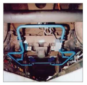
Railway Group Standard <u>GM/RT2477</u> "Track Circuit Assister Configuration for Rail Vehicles" sets out mandatory requirements for the provision and operation of TCAs.
