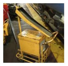
The manual method is the most widely adopted. Sand is normally supplied in 25kg
