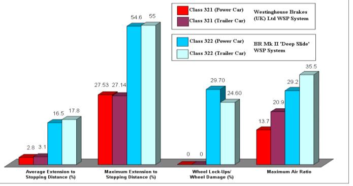
The graph shows significant performance improvements and reductions in wheel damage:
