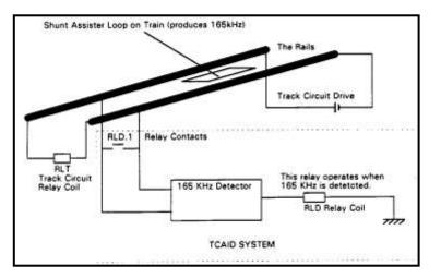
effect, the TCA clears the path so that the track circuit can operate properly.
