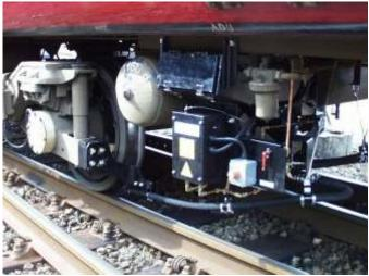
to enable sanding in brake step two and above with the ASD, or equivalent analogue brake settings. For tread braked units, the sander is triggered manually using a button on the cab driving desk.
