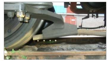
are manually controlled in both braking and traction because there are no WSP systems to automate the process. Retrofitting WSP to such units (<u>appendix A2.3.2</u>) would therefore allow automatic control of the sanding system as an added bonus.
