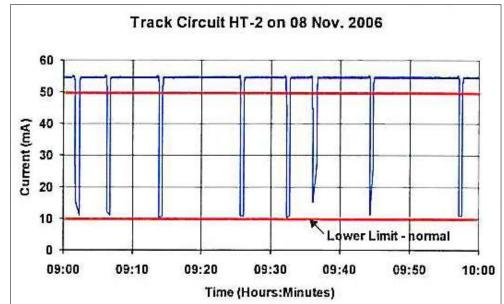
Threshold limits can be set to detect varying performance and enable track staff to react to emerging conditions and prevent a WSTCF occurring.
