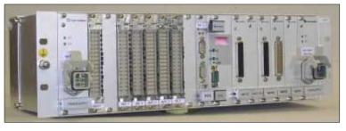
of significant wheel damage. WSP operates by modulating the brake actuators of slipping wheelsets, releasing and reapplying the brake at appropriate levels to maximise use of available adhesion. By controlling the speed of the wheelset to just below the forward speed of the train ('slip speed') a conditioning effect is seen which actually improves adhesion levels along the train as successive wheelsets condition the railhead.
