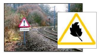
localised indication of poor railhead conditions by way of high intensity LED displays that are controlled from the signal box. The system comprises two constituent parts: the driver information signs and the signal box control console. Linking each of these devices is a radio communication network which allows information to be passed from one device to another completely automatically and securely, regardless of distance.
