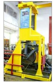
analysis of the three different leaf types (Horse Chestnut, Sycamore and Oak) validated the technique of leaf film creation using the full-scale wheel on rail rig;
