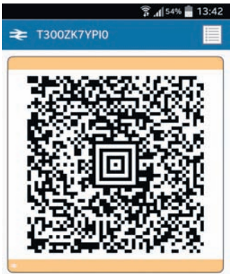
How an m-Ticket appears on the screen of a mobile device. The rectangular barcode contains digital data which defines the journey, fare, date and other details
