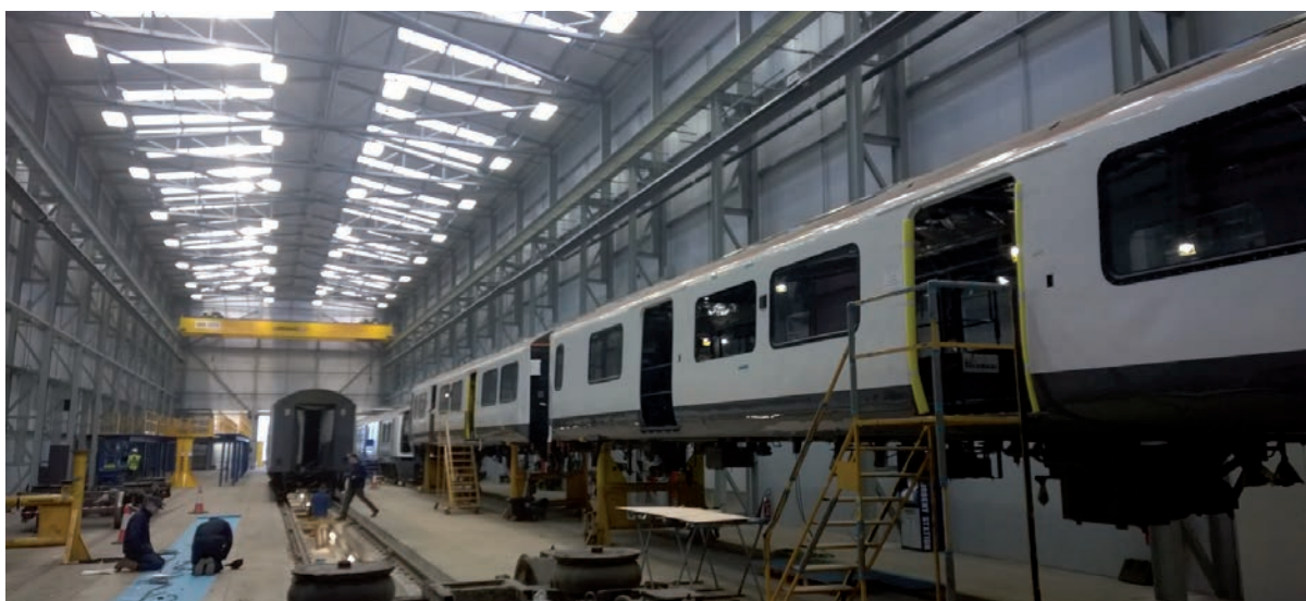
A BR-procured Abellio Greater Anglia Type E Class 321 EMU introduced in 1988, being life-extended to the 'Renatus' specification by Wabtec at Doncaster
