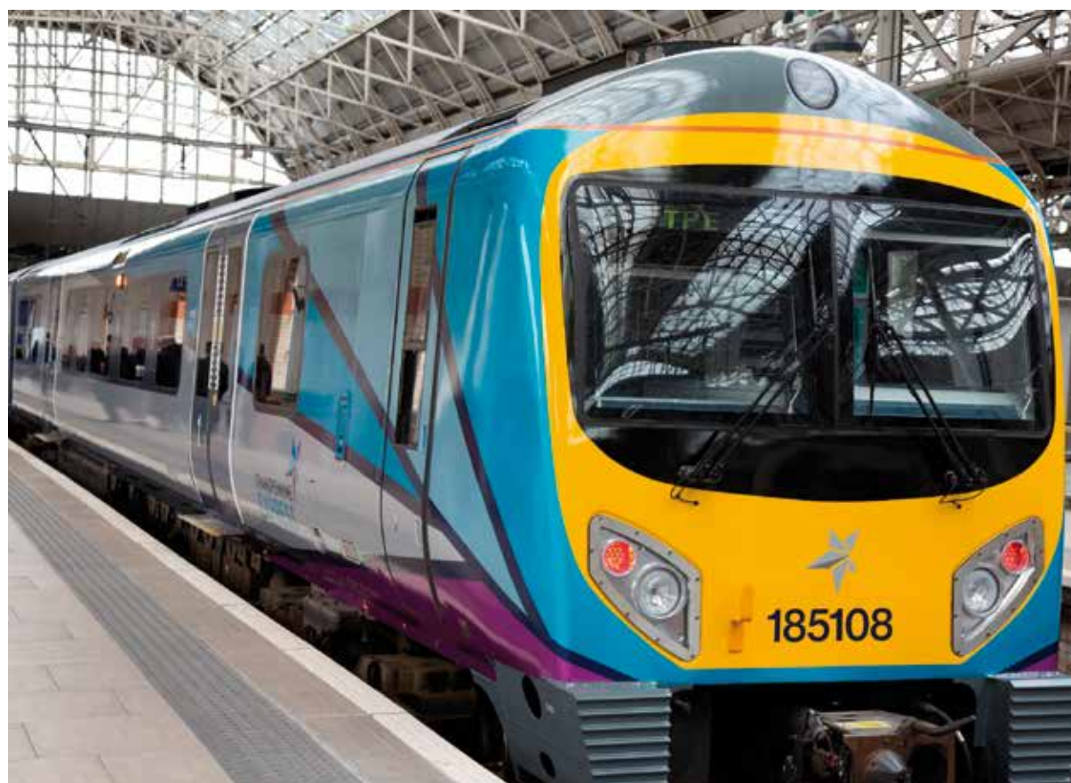
TransPennine Express Class 185 DMU. This is the diesel variant of the Siemens "Desiro" train, built in 2005.
