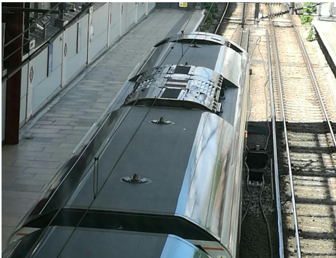
Figure 14: Class 700 roof showing antenna separation
