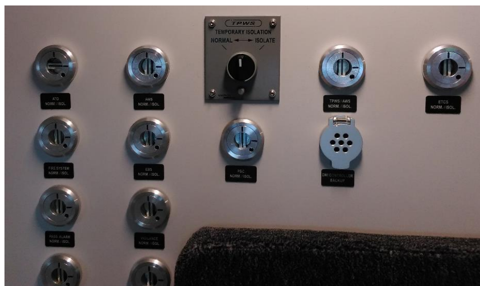
Figure 28: Isolation Switches on Thameslink Class 700
