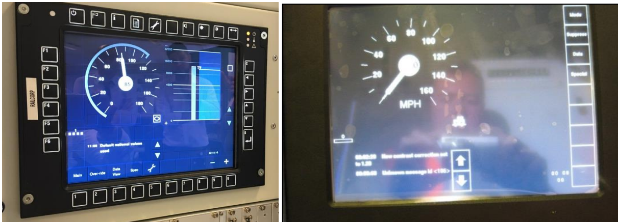
Figure 9: Examples of screen reflections on DMIs
