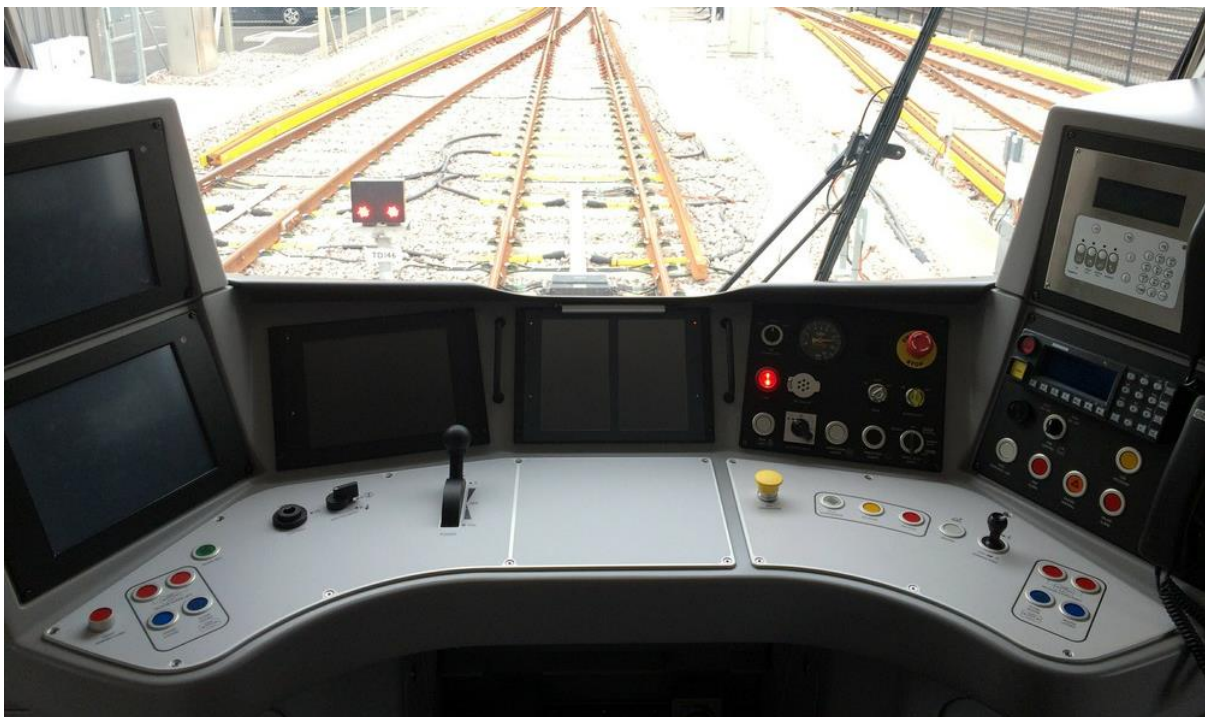
Figure 31: Class 700 at Three Bridges with Dual DMI shown
