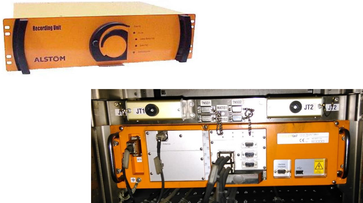
Figure 16: JRUs, including Alstom (top) and an Ansaldo JRU in situ on Class 158 (bottom)
