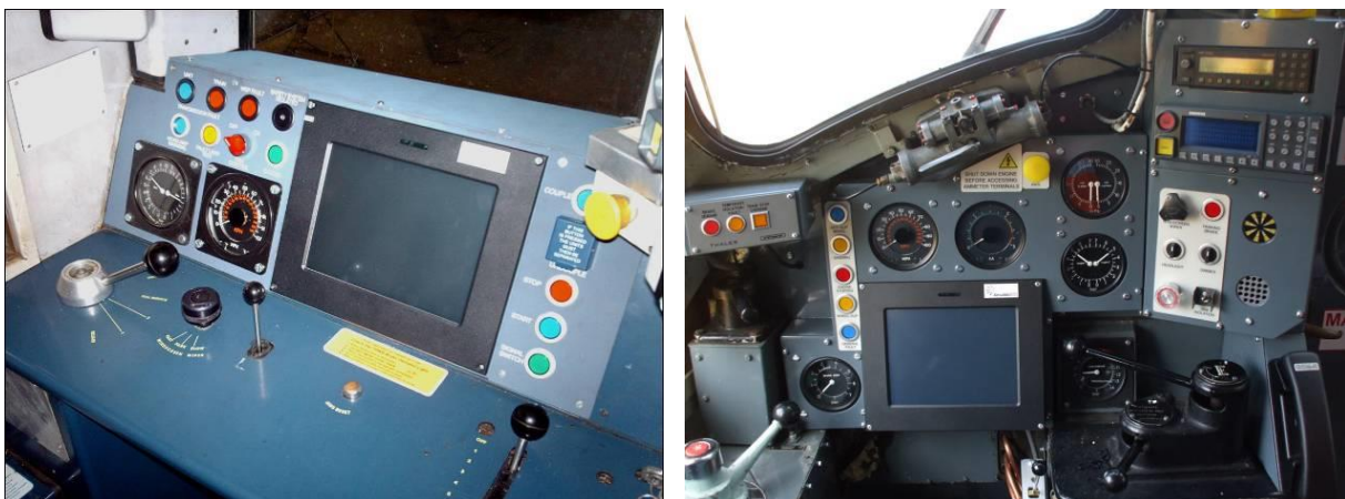
Figure 7: DMI fitment on Class 158 (left) and Class 97 (right)
