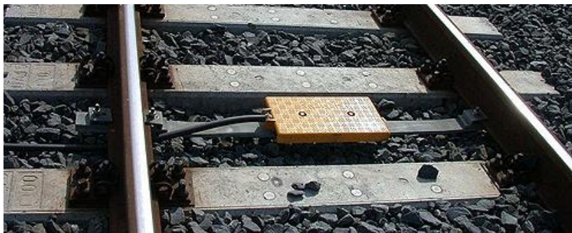
Figure 23: Example of Switchable Balise showing electrical connection to LEU
