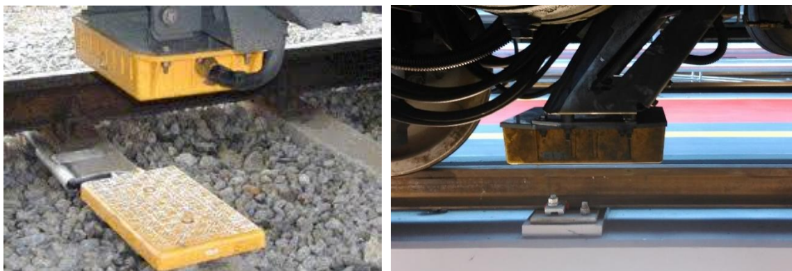
Figure 19: Example of 'air gap' interface between typical on-board Balise antenna and track-mounted Balise (left) and the Balise antenna as fitted on the Class 700 (right)
