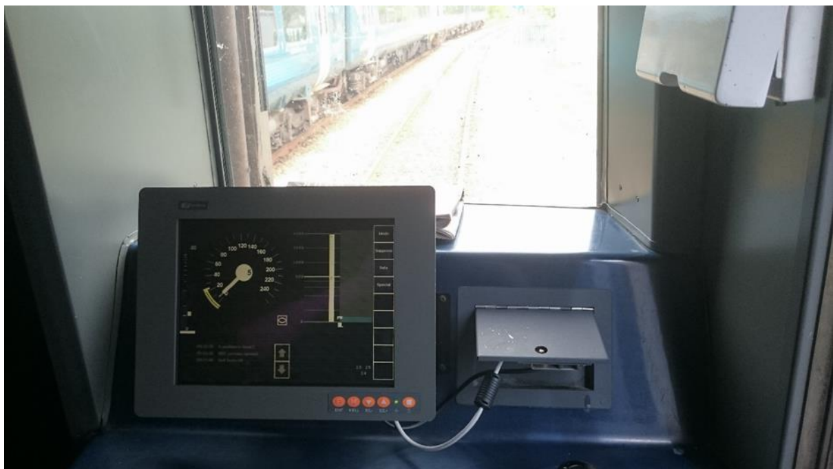
Figure 10: Mimic panel on the second man side of a Class 158 running on the Cambrian
