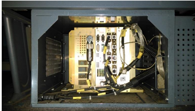
Figure 21: Under-seat mounted BTM on Class 158
