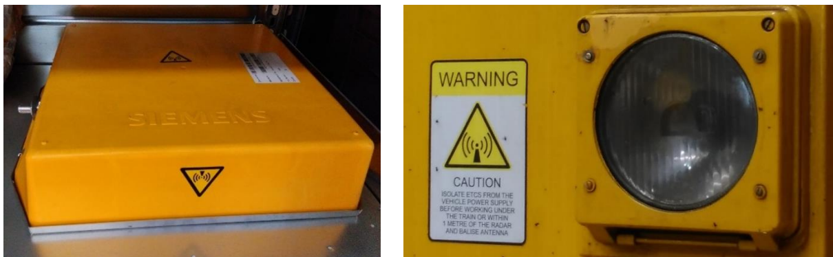
Figure 20: Examples of ETCS antenna safety warnings on a Siemens antenna (left) and on the front of a Class 97 locomotive (right)
