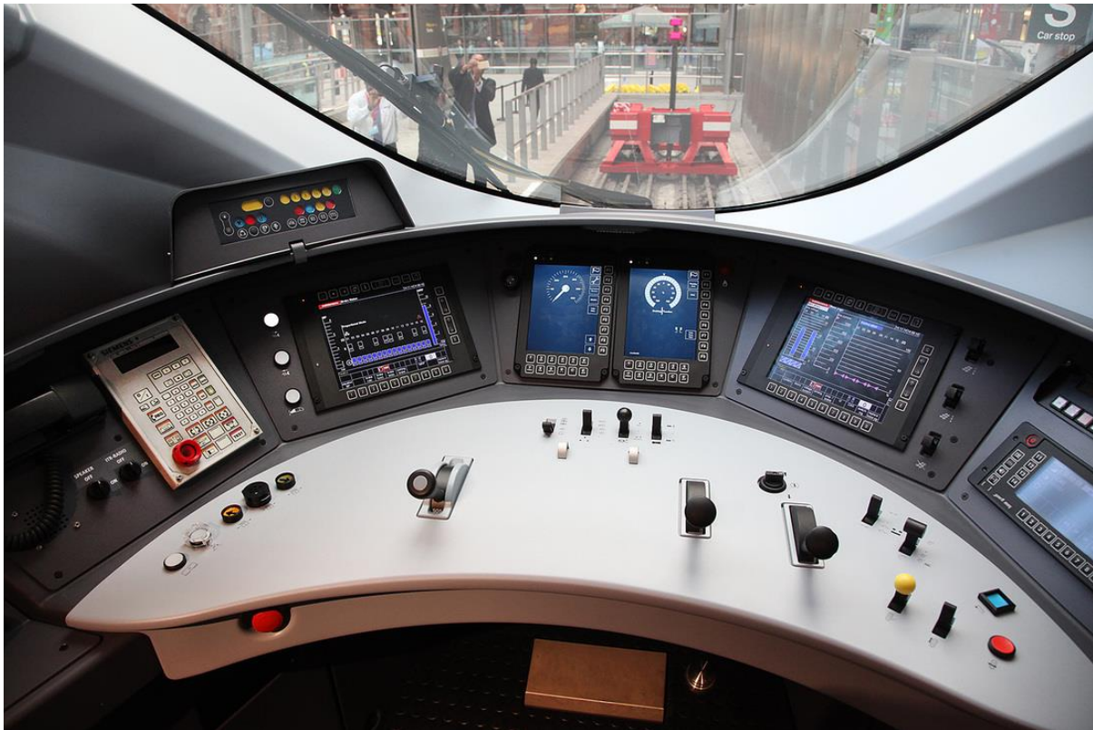
Figure 32: Class 374 (E320) with temporary TBL installation
