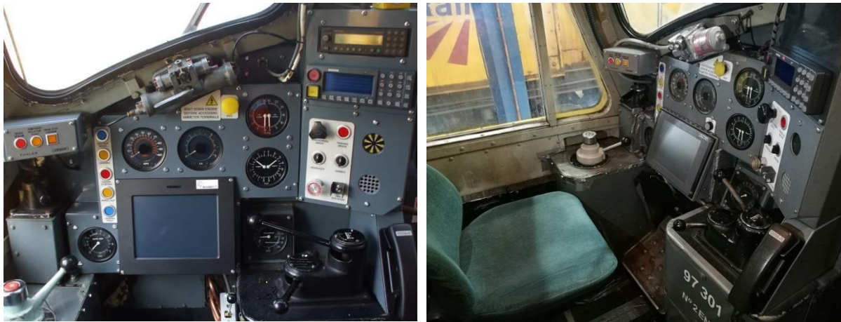
Figure 36: Class 37 (Now 97) Locomotive on Cambrian: Ansaldo fitment (left) and Hitachi (right)
