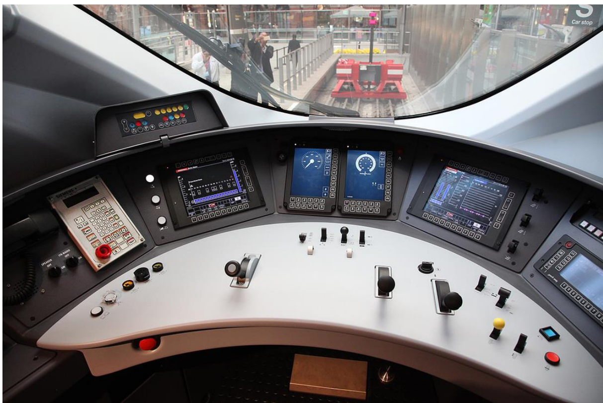
Figure 11: Eurostar DMI with European Systems Integrated via STM
