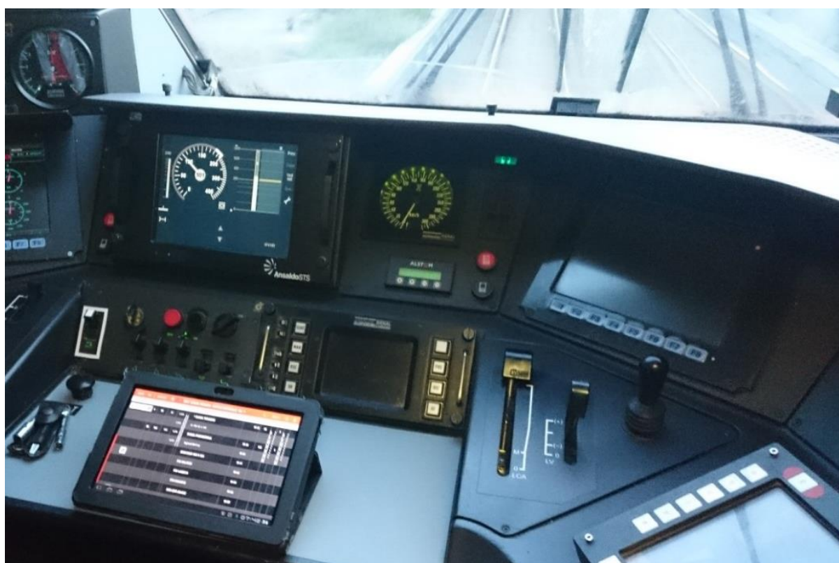
Figure 40: Italian High Speed Bombardier ERT500, highlights the separation between ETCS and their national system - SCMT
