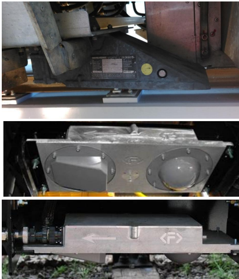
Figure 26: Examples of Doppler Radar: Deuta (top) and Faiveley (bottom)
