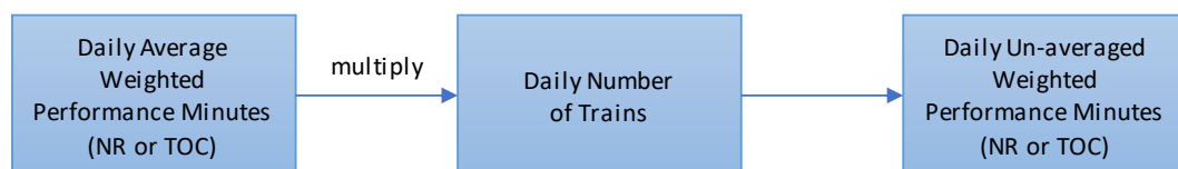
Figure A10.2: Calculation of daily un-averaged weighted performance minutes
